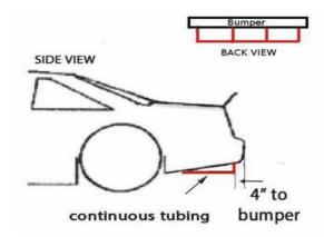
**3.4 FUEL LINES:** All fuel lines must be placed in a safe manner in the car. Mandatory fuel line safety valve OBERG SV-0828 or SRI Performance FPF-FSV must be used/installed as fuel exits the cell also check valve on vent required. Fuel filters mounted at rear of chassis must be located towards the center of the car. No plastic or glass filters permitted. Fuel must travel from the fuel cell to the carburetor and cannot pass into any performance enhancing devices.
