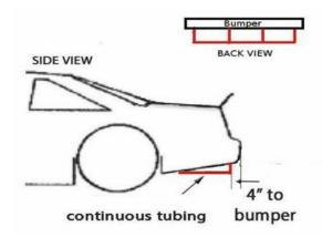
3.4 FUEL LINES: All fuel lines must be placed in a safe manner in car. Mandatory fuel line safety valve OBERG SV-0828 or SRI Performance FPF-FSV must be used/installed as fuel exits the cell also check valve on vent required. Fuel filters mounted at rear of chassis must be located towards the center of the car. No plastic or glass filters permitted. Fuel must travel from the fuel cell to the carburetor and cannot pass into any performance enhancing devices.
